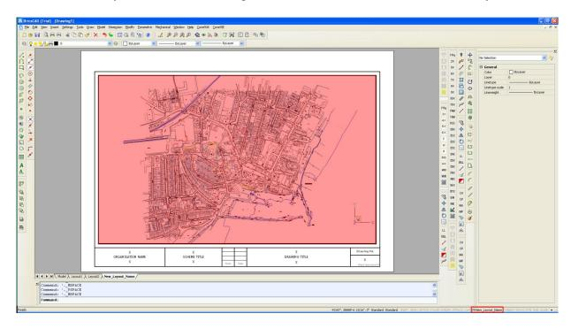
To switch between editing model and paper elements click on the layout label in the status barsurrounded by the red ring above – note: this is NOT the model or layout tabs. The label toggles between **M:New\_Layout\_Name** (for model entities i.e. the map & signs) and **P:New\_Layout\_Name** (for paperspace entities i.e. the title box and text)
