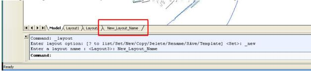
To switch to the layout view, simply click on this tab labelled "New\_Layout\_Name"
