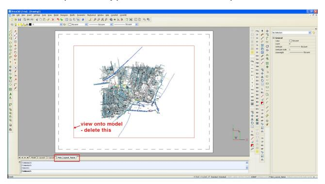
Here you can see the white A3 paper area, the limits the printer can output shown as the outer black dashed rectangle and the window onto the model view (the inner black rectangle).
