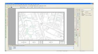
With the selector set to paperspace (**P:New\_Layout\_Name**) in the bottom right corner of the status bar, select the viewport that contains the view onto the model. This is NOT the drawing border of the title block, but a separate CAD entity – note the highlighted grips in the screen grab below.
