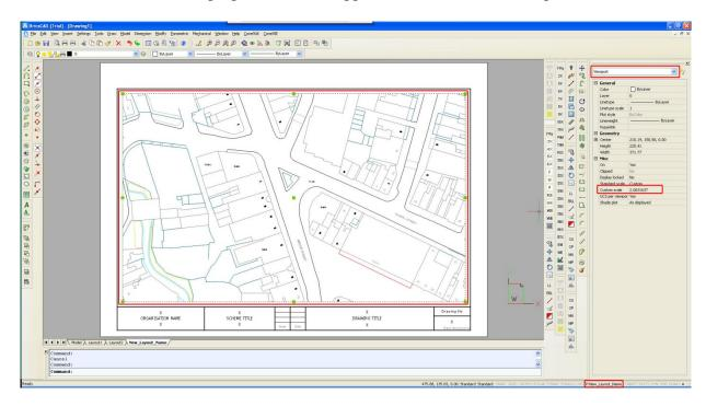
You can now set the Standard scale to one of the set values, or use the Custom scale highlighted. NOTE: as the drawing is in metres and the paper units are millimetres, there is a factor of 1000 difference, the current value of 1:1 is actually 1 plotted millimetre to 1 drawing unit (metre) or rather 1:1000
