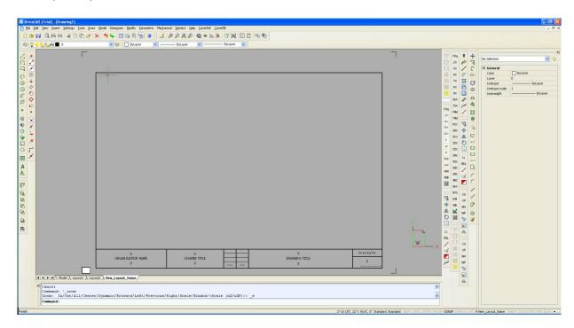
You may notice the drawing border no-longer fits the white paper (shown in the bottom left corner), this is due to incorrect printer settings – normally inches rather than millimetres.
